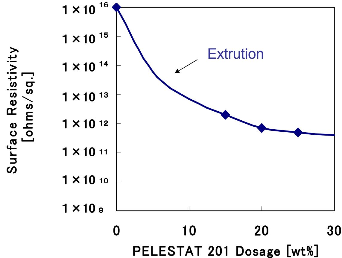
Figure 1 Surface Resistivity v.s. Dosage [23°C(73F), 50%R.H.]
