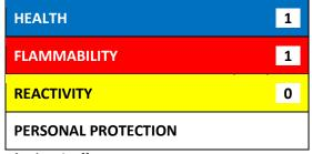
Caution: HMIS® ratings are based on a 0-4 rating scale, with 0 representing minimal hazards or risks, and 4 representing significant hazards or risks. Although HMIS® ratings are not required on SDSs under 29 CFR 1901.1200, the preparer may choose to provide them. HMIS® ratings are to be used with a fully implemented HMIS® program. HMIS® is a registered mark of the Nation Paint & Coatings Association (NPCA). HMIS® materials may be purchased exclusively from J.J.Keller 800-327-6868.
